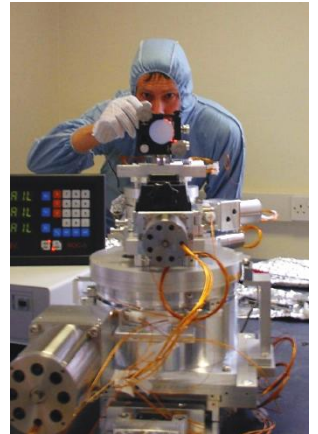
Testing diamond crystal goniometer
