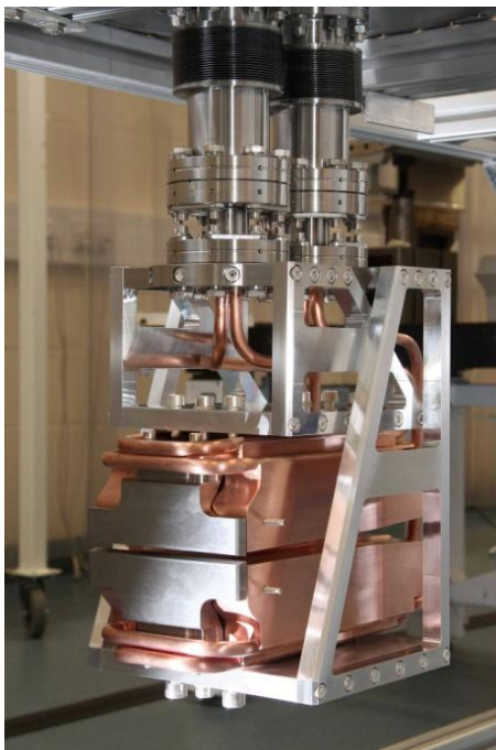
Above: Australian Synchrotron Imaging & Medical beamline - horizontal & vertical slits, & 5-axis multi-filter system.
