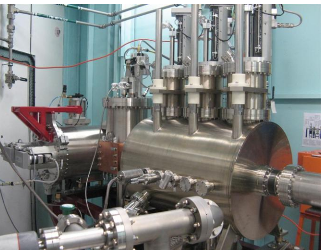
Above: Australian Synchrotron Imaging & Medical beamline - horizontal & vertical slits, & 5-axis multi-filter system.
