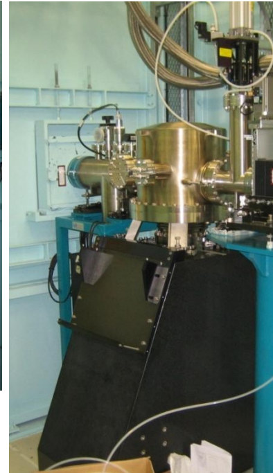
Above: Secondary Source Aperture installed on ID5 Micro-Spectroscopy beamline at the Australian Synchrotron.
